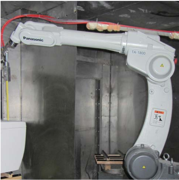
Robot glazing line
