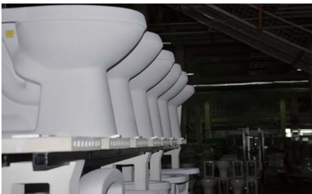
Kiln loading area
