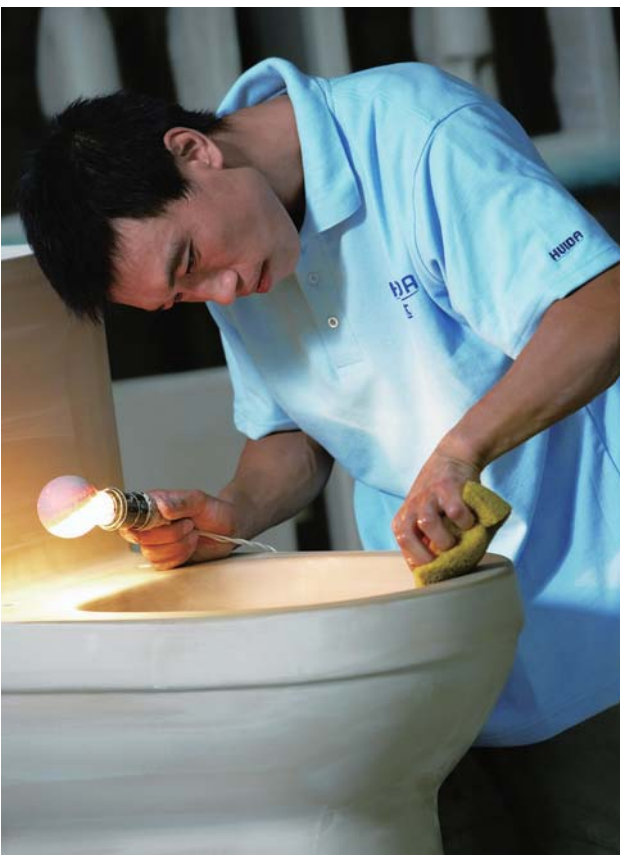
Inspection of semi-finished products
